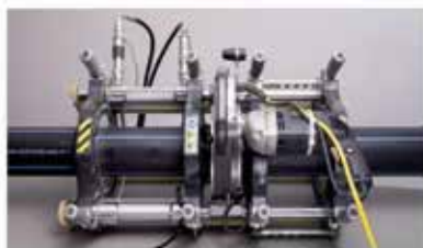
Mill the parts to be welded and check the alignment.
