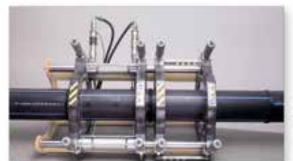
Stage 5 welding with element in pressure
